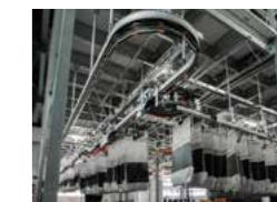
Pocket Sorter™, a hanging high-speed sorting system
