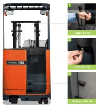
To prevent unintentional operation, battery is reached out only when 1, 2, and 3 are operated simultaneously.
