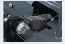
**Tilt Cylinder Boots** Each boot covers the exposed portion of the rod for the tilt cylinder, protecting it and the oil seals.
