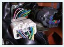
Water-Resistant Connectors Connectors for most electrical components are highly water-resistant, increasing the reliability of the electrical system.
