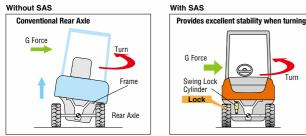
An onboard computer monitors the movement of the forklift and locks the swing of the rear axle when necessary, such as during turns.
