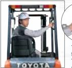
The seat swivels to the right to facilitate operation in reverse. The seat also swivels to the left to make it easier to enter and exit
