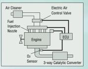
Electronic control is used on the 4Y engine to regulate the fuel injection and ignition systems. This is combined with the 3-Way Catalytic Converter System to filter out carbon monoxide (CO), hydrocarbon (HC) and nitrogen oxide (NOx) gases.
