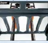
The overhead guard, mast and instrument panel have been designed to provide excellent visibility of the fork tips at the most frequently used lift heights.
