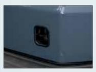
Hood Latch The easy-to-operate latch provides quick access to the engine compartment.
