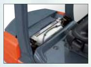
**Radiator Cover** No tools are needed to remove the radiator cover. The fasteners can easily be turned by hand to enable quick inspections or servicing.
