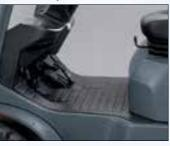
The ORS seat can be adjusted 150 mm forward and backward to provide comfort and support to almost all sizes of operators. \*ORS: Operator Restraint System
